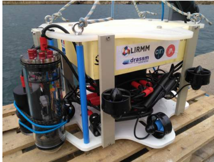
FIGURE 6.3: The Remotely Operated Vehicle Dumbo and the acquisition system A, used to record the harbor sequences.
